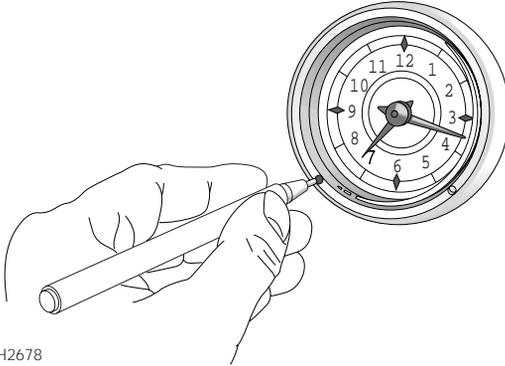
To adjust the time, use a ball point pen or similar probe to advance or put back the time, using the right or left hand buttons at the bottom of the clock bezel.
