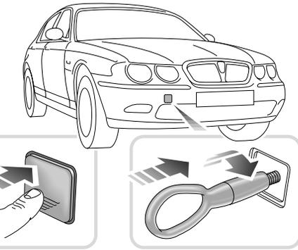
Your car is equipped with a fixed towing point at the rear of the car and a removable towing eye at the front. The front towing eye is stored in the tool kit beneath the boot floor when not in use.
