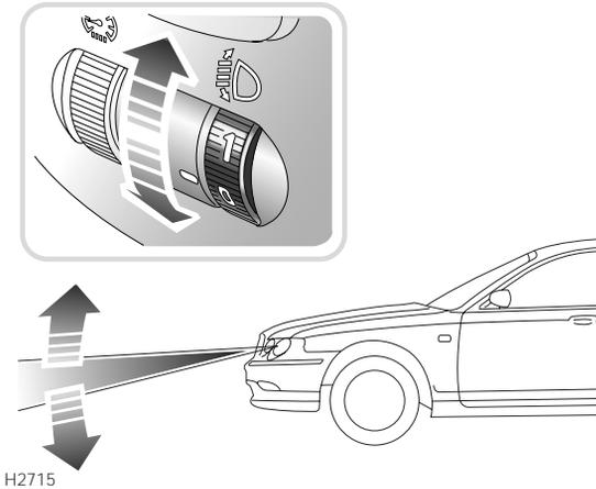
The angle of the dipped beams is affected by the distribution of passenger and luggage weight within the car. It is important that the headlights are adjusted to ensure that the point at which they meet the road surface provides adequate illumination ahead of the vehicle, without dazzling other road users.
