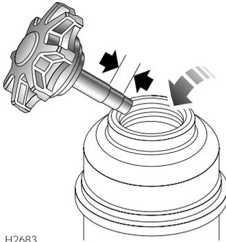
Check the fluid level every week. The engine should be switched off with the system cold and the front wheels in the straight ahead position before the level is checked.
