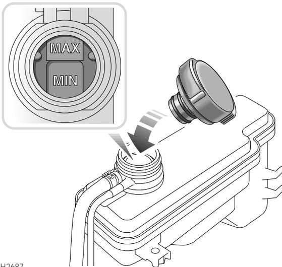
If the level is below the 'MAX' mark, top-up with a 50% mix of water and ethylene glycol based anti-freeze (containing no methanol) with Organic Acid Technology (OAT) corrosion inhibitors (see 'Anti-freeze').
