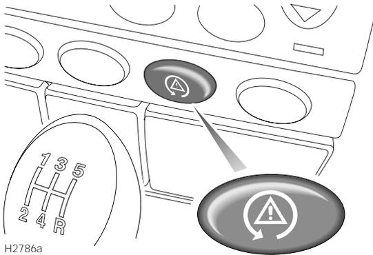
Traction control is entirely automatic in operation. However, the system can be manually overridden by pressing the traction control disable switch (see illustration). The system will then remain disabled until the switch is pressed a second time, or until the starter switch is turned off.
