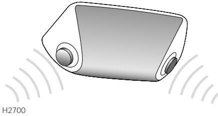
Interior space protection (ultrasonics) is designed to protect the interior of the car from intrusion (entry by a thief through a smashed window, for example). A pair of ultrasonic sensors monitor the interior space and activate the alarm if air movement is detected in the passenger compartment.
