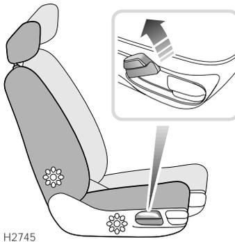
Ensure the seat is occupied before adjusting the height. Lift the lever and apply weight to lower the seat rearwards, or allow the seat to rise forwards, as required.
