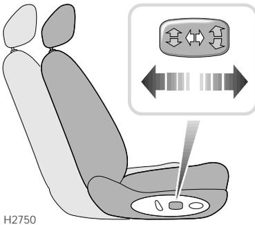
Push and hold the switch forwards or rearwards to move the seat to the desired position.
