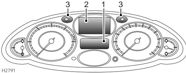
The standard instrument panel features two main clusters of warning lights, one situated in the centre of the pack (1) and the other located at the upper centre of the instrument pack (2).
