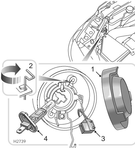
1. Remove the rubber cover from the rear of the headlight.
