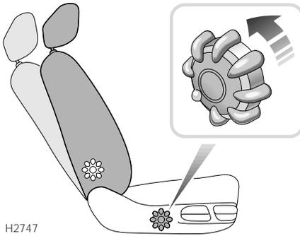
Rotate the handwheel to adjust.
