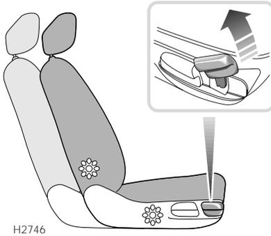
Lift the lever and slide the seat into position. Make sure the seat is locked in position before driving.
