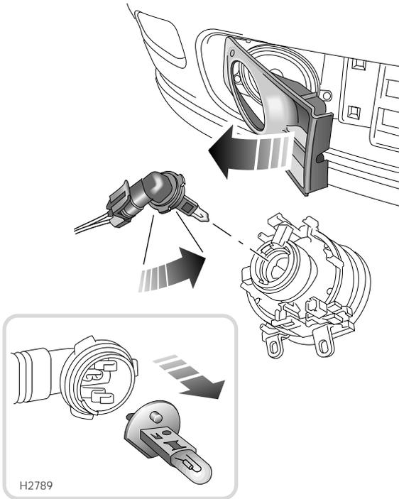
Pull the inboard side of the fog light surround away from the front of the car – see illustration (gentle leverage using a flat-bladed screwdriver behind the surround may be necessary).
